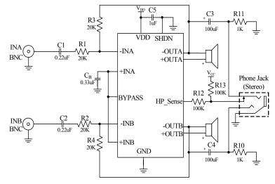
Figure 1. Typical Audio Amplifier Application Circuit
